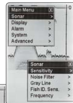
▶ The Noise Filter function reduces the undesired signals that come from your boat engine, turbulence or electrical sources.
